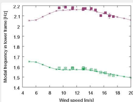
*A comparison between HAWCStab2 predicted and measured frequencies of the edgewise rotor whirling modes of a 2750 kW turbine during operation.*
