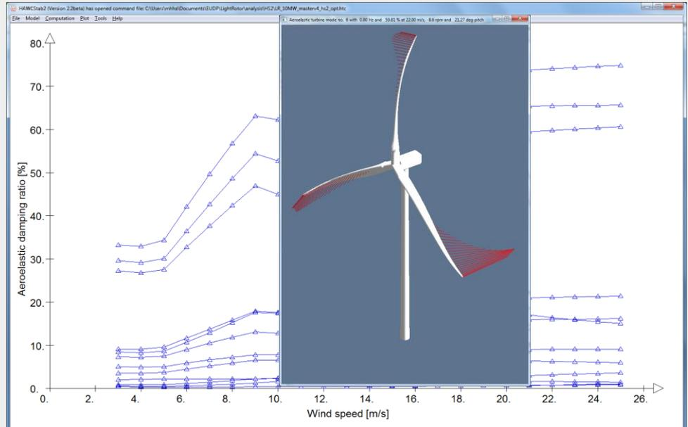
*The graphical user interface of HAWCStab2 shows a calculation of aeroelastic damping for a wind turbine versus operational wind speed. A click on a point in this diagram starts an animation of the corresponding mode shape including unsteady aerodynamic forces.*
