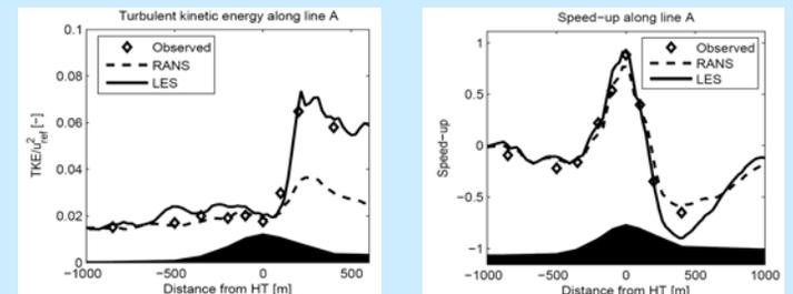
LES and RANS results. Turbulence intensity (left) and Speedup (right).
