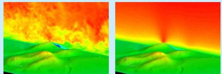
Instantaneous velocity contours of the wind over the Askervein hill using LES (left) and RANS (Right). LES gives detailed information of the turbulent wind; However, the computational cost is high.
