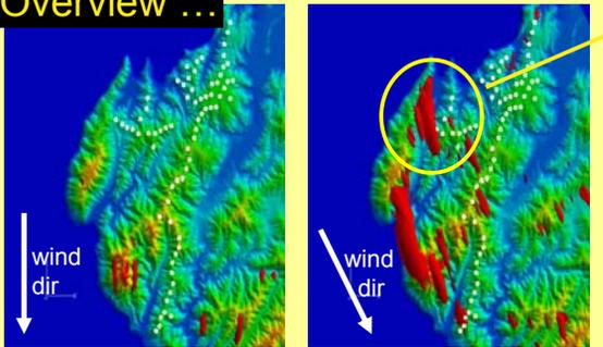
CFD results from a complex site showing regions of high turbulent kinetic energy for two wind directions.
