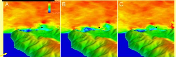
Vertical plane showing contours of wind speed at three incidences (A→B→C) - wind is from left. The color code from high to low speed: Red, yellow, green, blue. The black dot symbolizes a wind turbine.
