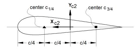
Figure 5: Illustration of aerodynamic centers c1/4 and c3/4
