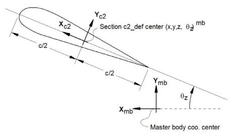
Figure 2: Illustration of c2\_def coordinate system related to main body coordinates.
